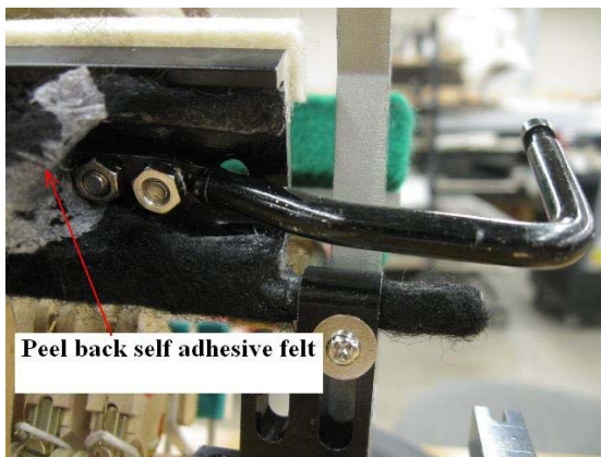
Illustration 26 & 27 – Actuation Lever adjustment (Rear and Front view)
