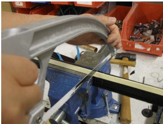
Illustration 7 – Cutting mute rail breaks
