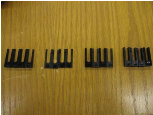
Illustration 20 & 21 – Assorted mute rail spacing shims
