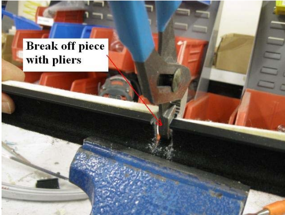
Illustration 9 – Removing break area
